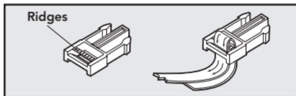
The ridges must be facing up; the collar will slip if it is not properly threaded.
