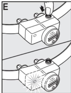
level 6 will cause the Receiver Collar to revert to level 1. Refer to the Function and Response Table to choose the Static Correction level that best fits your pet. The Receiver Indicator Light acts as a low battery indicator. The light will flash every 4 to 5 seconds when battery replacement is required.
