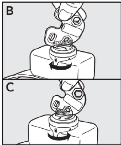
To remove the battery, turn the battery counter-clockwise using the edge of the Test Light Tool (C). **DO NOT** attempt to cut into or pry open the battery. Be sure to discard the used battery properly.
