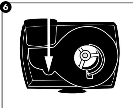
6. Remove the teardrop shaped stator by pulling up on the small lip.
