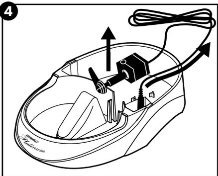
4. Remove the pump from the square indentation and pull the in-line plug up through the hole.
