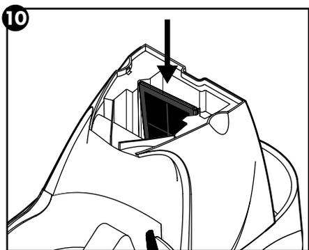
10. Rinse the carbon filter and insert it into the housing. It fits narrow side down, and the black side faces the front.
