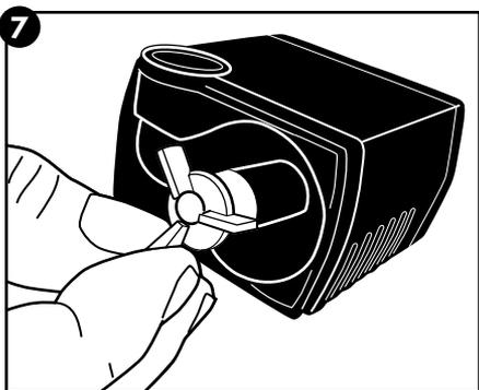
7. Use a fingernail to pull out the impeller, which is held in place magnetically.
