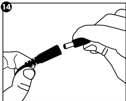
14. Make sure the electrical power cord, the adapter and your hands are completely dry. Connect the in-line plug and make sure no silver is showing, then plug the adapter into a standard electrical wall outlet.
