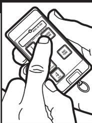
Press GOOD Tone button on the transmitter within 30 seconds of installing receiver battery. The components now work together.
