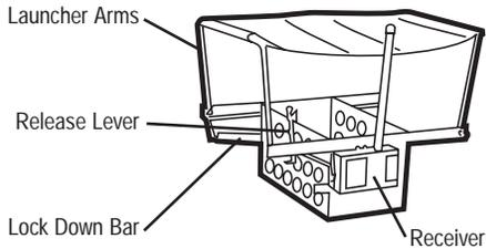
**Manual launcher:** Attach a pull cord (you provide) through the Pull Hole, and then to the bottom hole of the Release Lever. Pull the cord to release the launcher.
