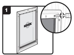
Slightly loosen screws from interior frame of pet door.
