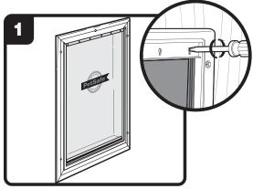
Remove screws from the interior frame of pet door.
