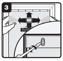
Replace vinyl flap and metal bar. Now, adjust flap horizontally and/ or vertically to fit into door frame and tighten when correct.
