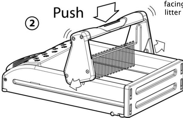
Ensure rake handle is facing the front of the litter box as shown in illustration
