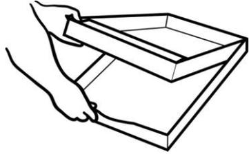
**Step 2:** Lower litter box onto litter tray. Listen for a click. This means the magnets on the waste trap lid have connected with the magnets on the litter tray. Make sure the sides of the litter box are flush with the sides of the litter tray.
