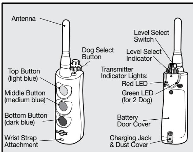
**Level Select Switch:** Provides multiple levels of Stimulation. *Note: When set to Level "0", the LED's on the Receiver Collar will still light up but no correction will be delivered.*
